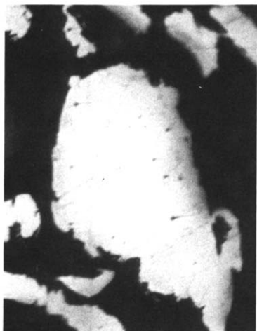
Fig. 2. Al-Li alloy before hydridation.
